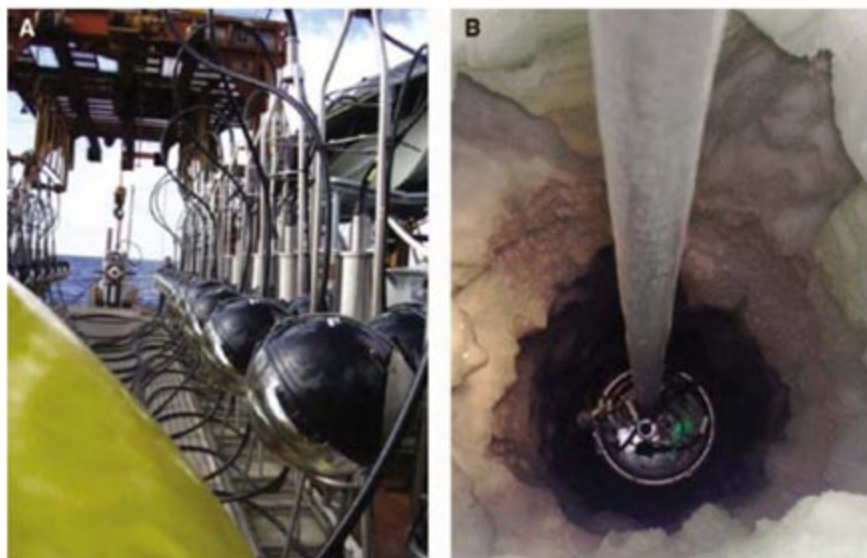
Fig. 2. Deployment of optical sensors (10-inch photomultiplier tubes encased in a centimeter-thick glass pressure housing) by ANTARES in water (A) or by IceCube in (temporarily melted) ice (B).
